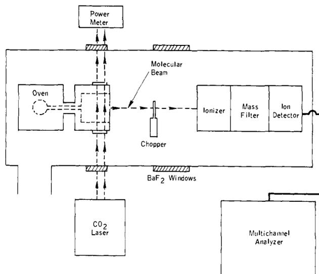
**Figure 5.** Schematic diagram of the experimental apparatus used in the photofragment identification experiments.
