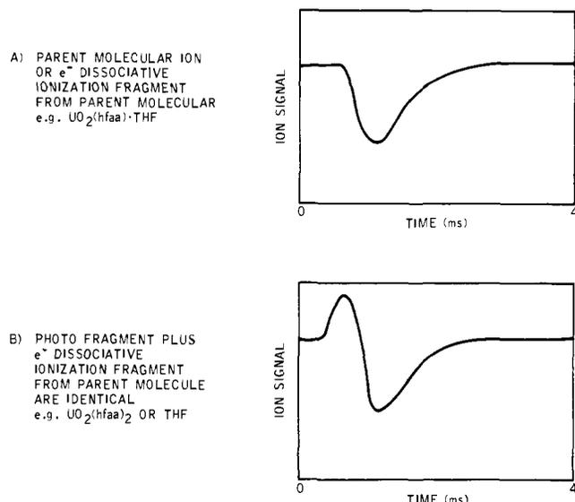
**Figure 6.** Typical time-of-flight responses for the parent molecular ion (A) and for a fragment ion (B). The fragment ion signal arises from two sources: one is the fragment produced by the dissociative ionization of the parent molecule (negative going signal) and the other ion is due to the directly produced photofragment (positive going signal and shorter TOF).
